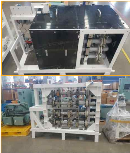
HYPOCHLORITE GENERATION UNIT
